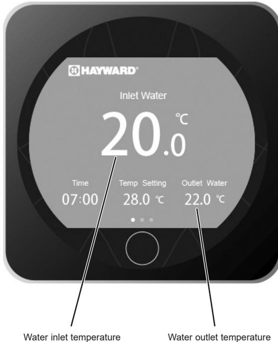
Note: Opening the by-pass valve creates a weaker flow, which leads to an increase in  $\Delta T$ .
