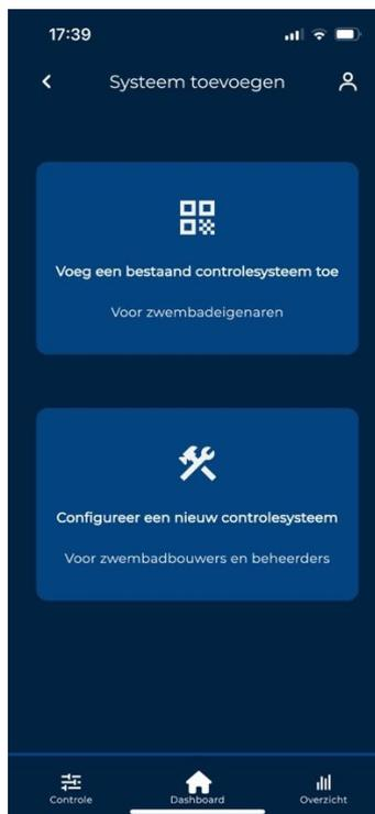
The configuration proceeds in 3 steps. In the first step, you scan the code present on the Wattr module. If scanning does not succeed, you can always enter the code manually; the text lights up when the Wattr module is known and the code is correct. Next, enter the name of the installation, which is visible when using the app, and the location of the pool. (A correct location is necessary for using weather data).
