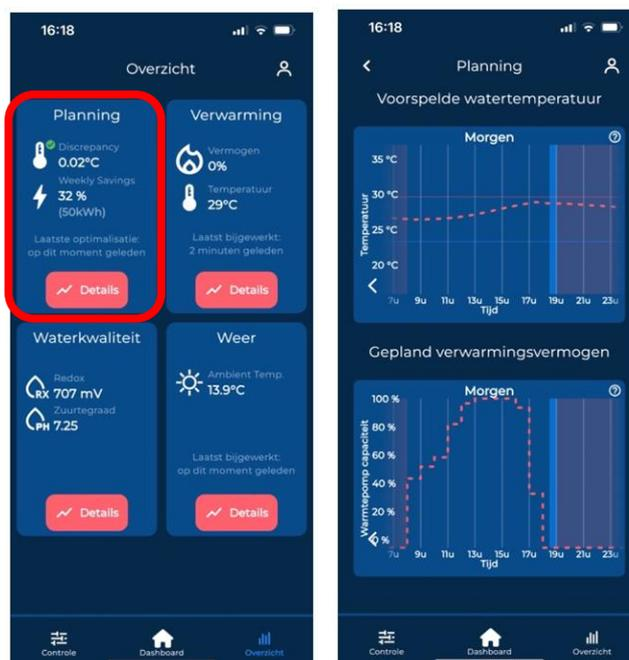
When viewing the forecast graphs, the scheduled swimming moments are coloured light blue, the predicted water temperature and heat pump running capacity are indicated by red dotted lines.
