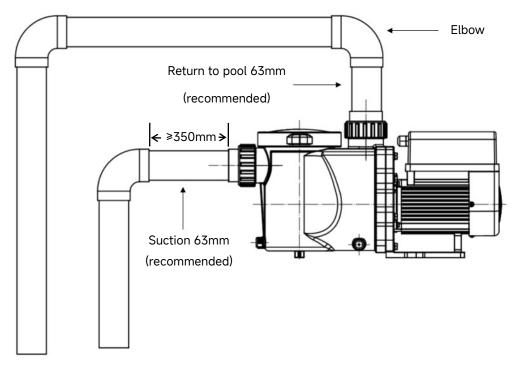
Figure 2 - Plumbing and Fittings installations
