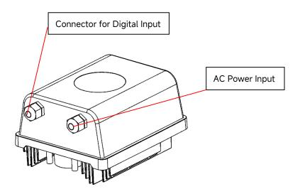
Figure 4 - Connector port location
