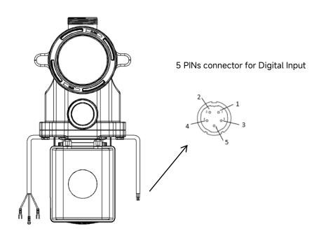
Figure 5 - Digital Input connector
